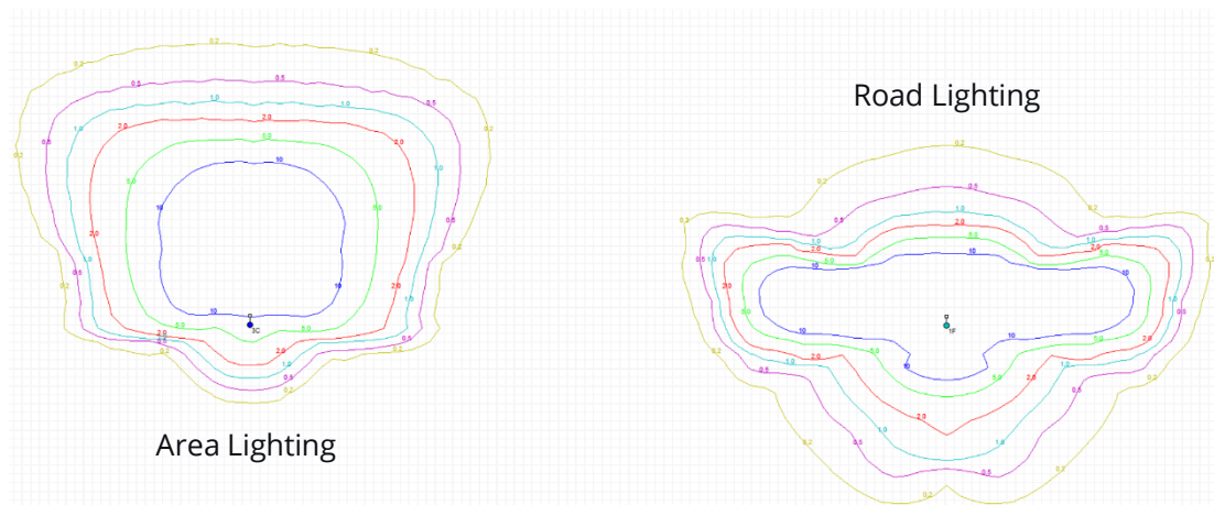
Figure 12: Example of Two Different Luminaire Optics
